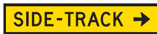
SIDE-TRACK LEFT OR RIGHT ARROW (L or R) T5-2A 1200 x 300 T5-2B 1800 x 450
