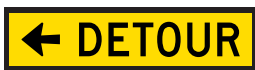
DETOUR LEFT OR RIGHT OR UP ARROW (L or R or UP) T5-1A 1200 x 300 T5-1B 1800 x 450
