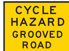
CYCLE HAZARD GROOVED ROAD T2-207A 1200 x 900
